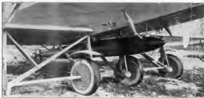
UNDERCARRIAGE OF THE GLENN MARTIN TORPEDO PLANE, WITH A 1500-Lb. EMERGENCY NAVY TORPEDO IN PLACE
